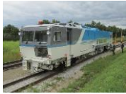
Plasser Multiple Tie Tamper, etc
